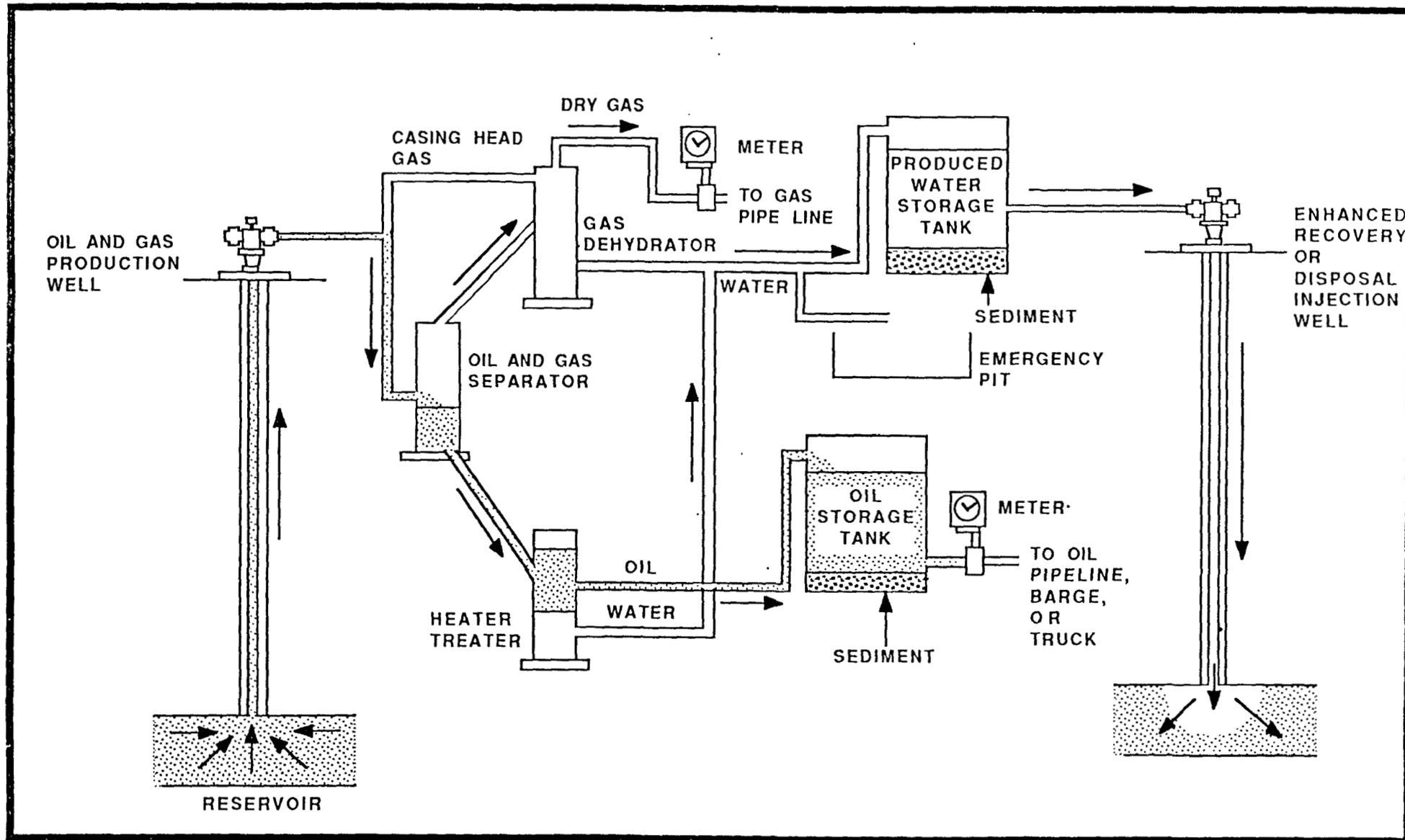
Figure II-3 Oil Production With Average H<sub>2</sub>O Production With Dissolved/Associated Gas
