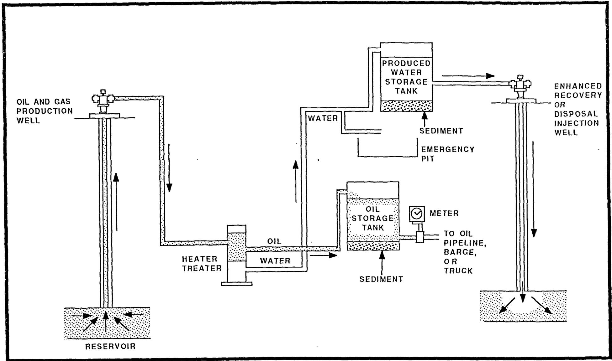
Figure II-4 High Oil/H<sub>2</sub>O Ratio Without Significant Dissolved/Associated Gas
